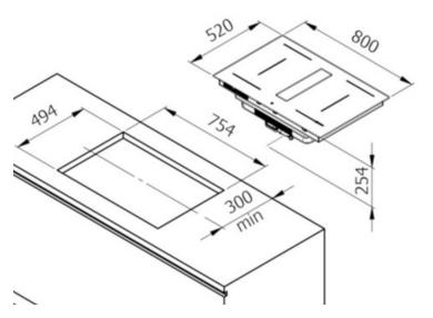
The worktop must be a maximum of 40 mm thick to ensure sufficient exhaust air.
